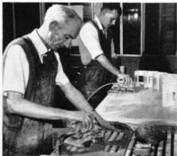
ABOVE: Tony Palmer of Spray shop, masking a strip on the insides of parts so that earthing connections can be made. Tony paints in his spare time, and two pictures of his are on the wall
