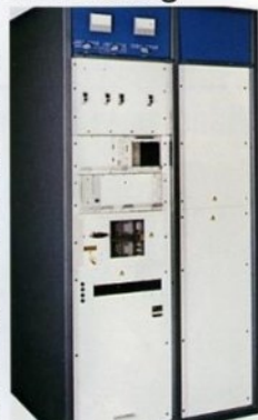
The 20kW transmitter.
