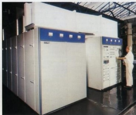
A B6127 transmitter under test at the Chelmsford development laboratories.
