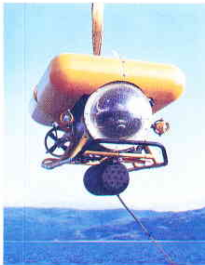
Minnow, a remotely controlled vehicle developed by Marconi Underwater Systems for the new generation of mine countermeasures vessels. Small but powerful, it investigates underwater contacts by TV, sonar and camera destroying mines it locates by placing charges.
