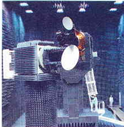
Antennae for satellites being tested in Marconi's Space Systems' antenna test range, Portsmouth.
