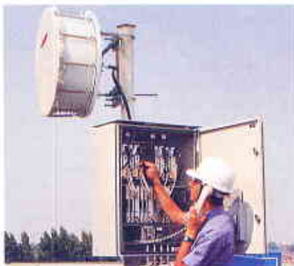
Pole mounted digital radio equipment made by GEC Telecommunications which meets the needs for voice and data links across cities.
