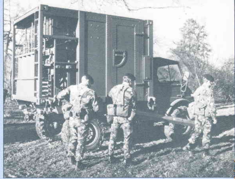
ISOLATOR shelter fitted with military radio equipment by MSRL.
