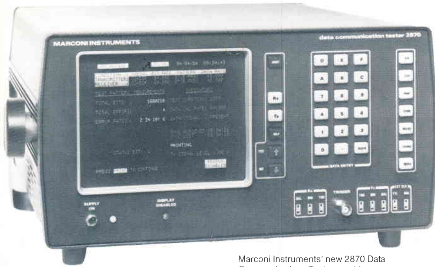
Marconi Instruments' new 2870 Data Communications Tester combines a comprehensive pattern generator and error detector to allow tests on lines operating from 50 bit/s to 128 kbit/s.
