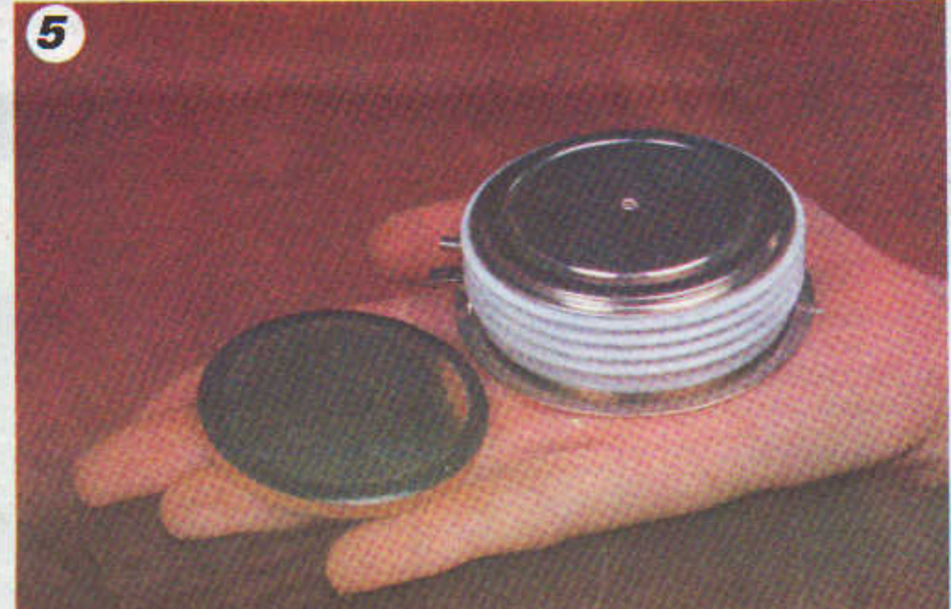
A 56mm thyristor and basic unit, manufactured by Marconi Electronic Devices. 12,000 of these were used in the Cross Channel link.
