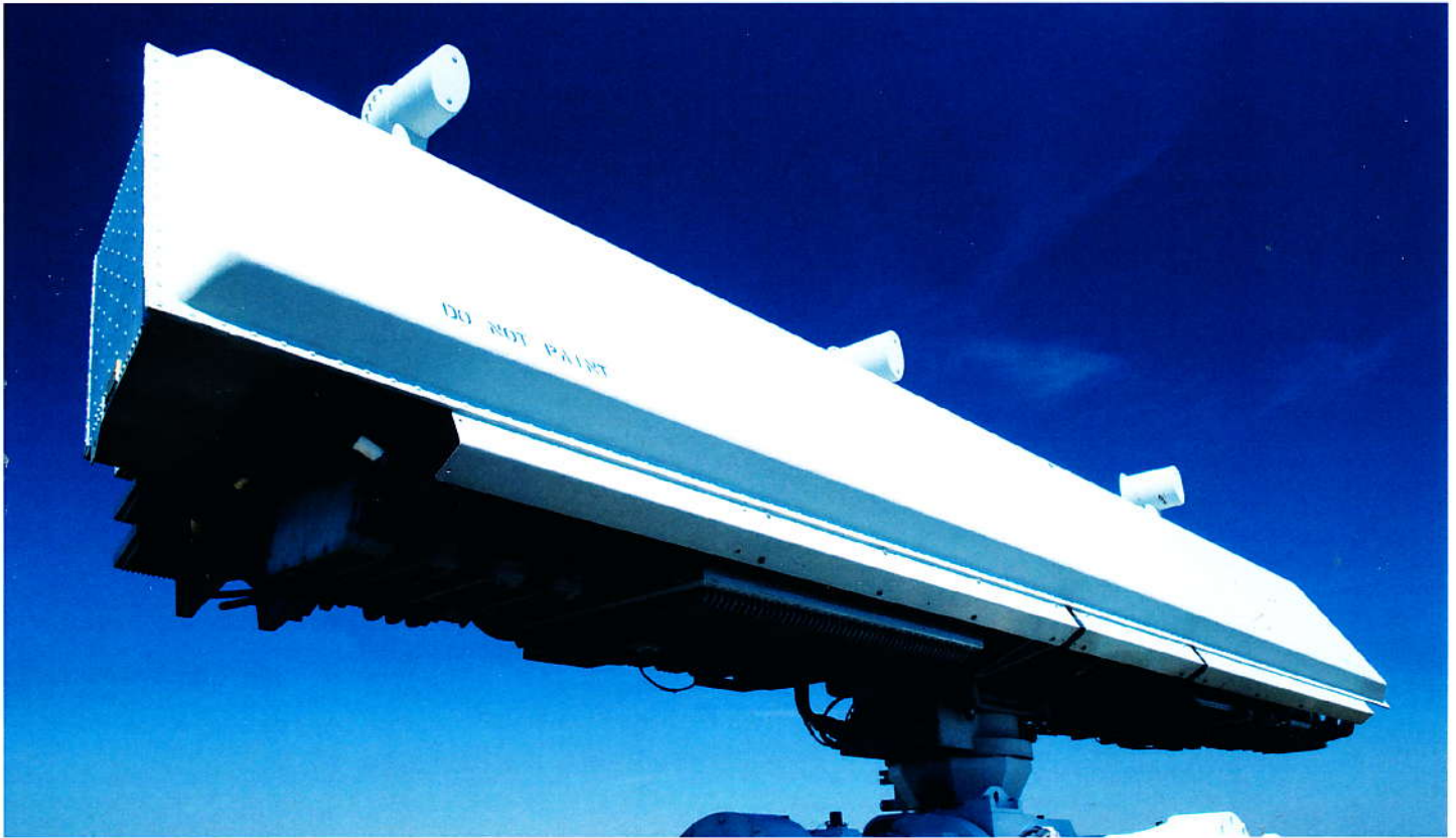
Above: the Type 996 radar
