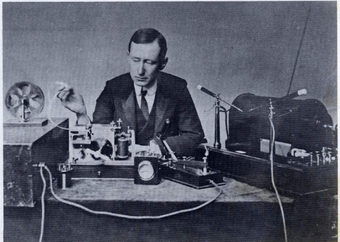
Marconi with 1902/3 wireless apparatus. On the right is the 10" induction coil spark transmitter, on the left the coherer receiver, and in the centre the Morse inker and 'grasshopper' key.
