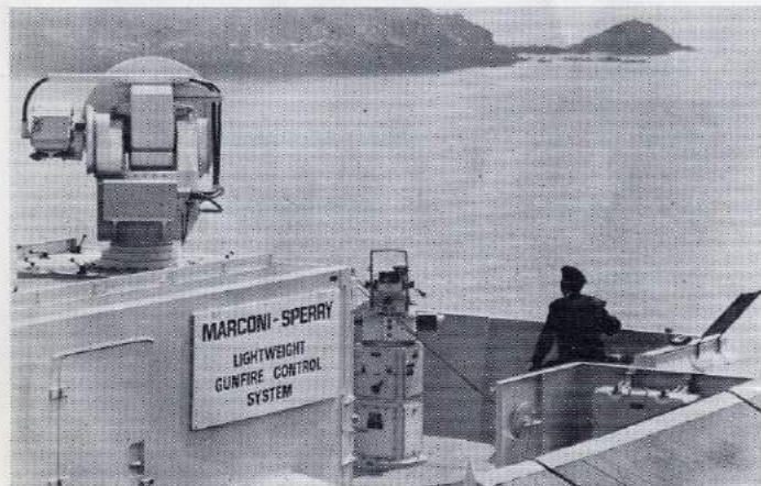
The Marconi ST802 radar director on the Royal Navy's gunnery range at Wembury, near Plymouth, during live firing trials at air and surface targets.
