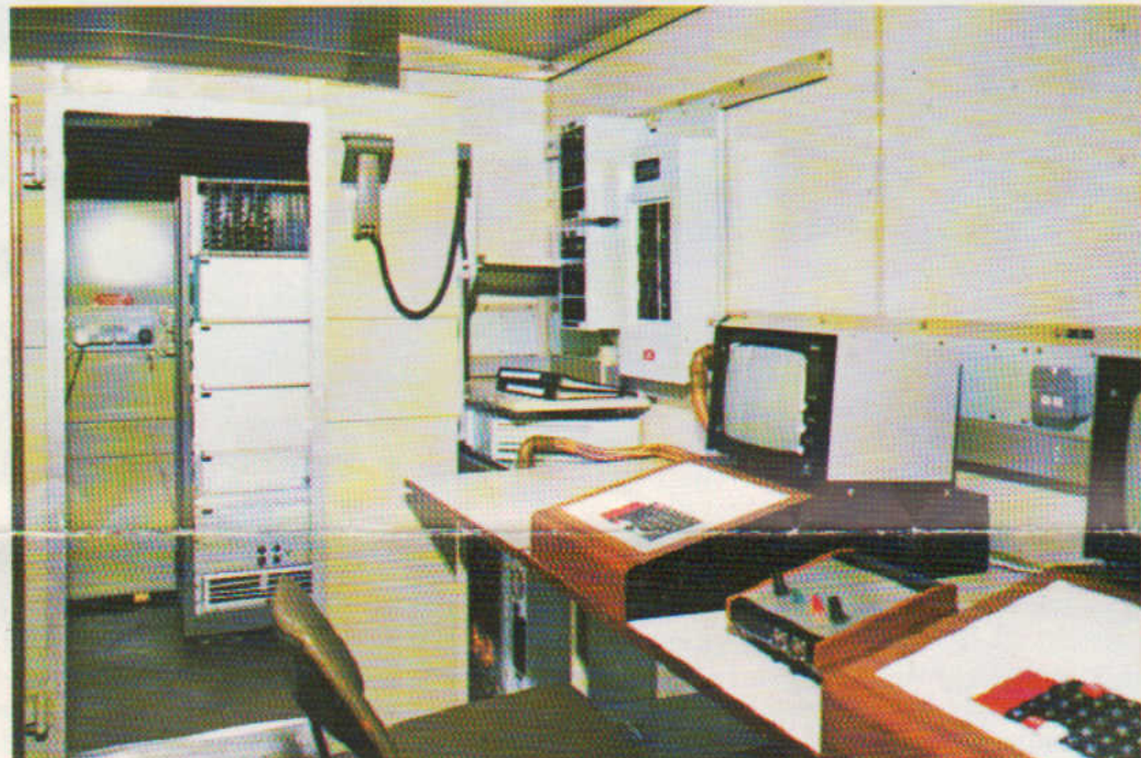
Simulator cabin showing aircraft control units and peripheral equipment cabinet
