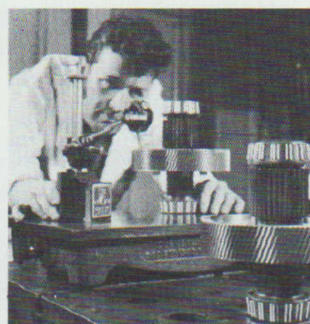
Checking gearbox components
