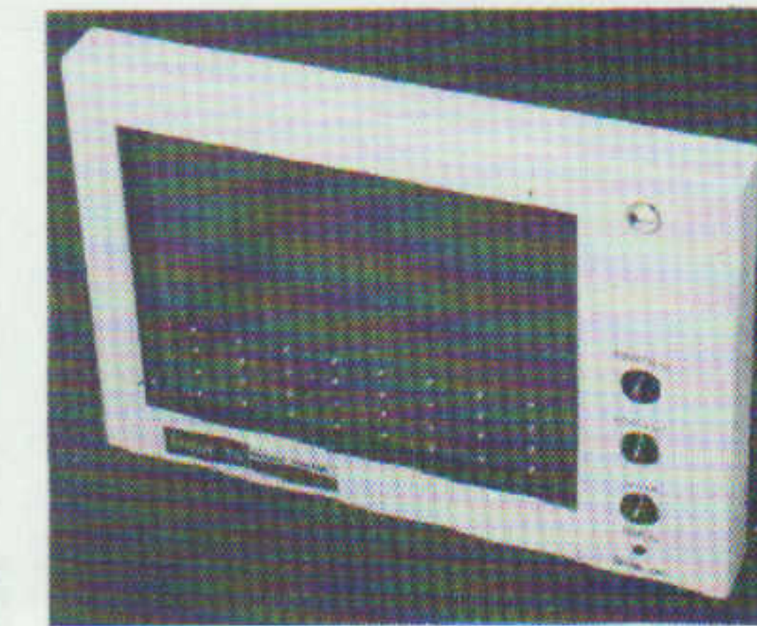
Marconi Digilux touch sensitive display, showing location studs
