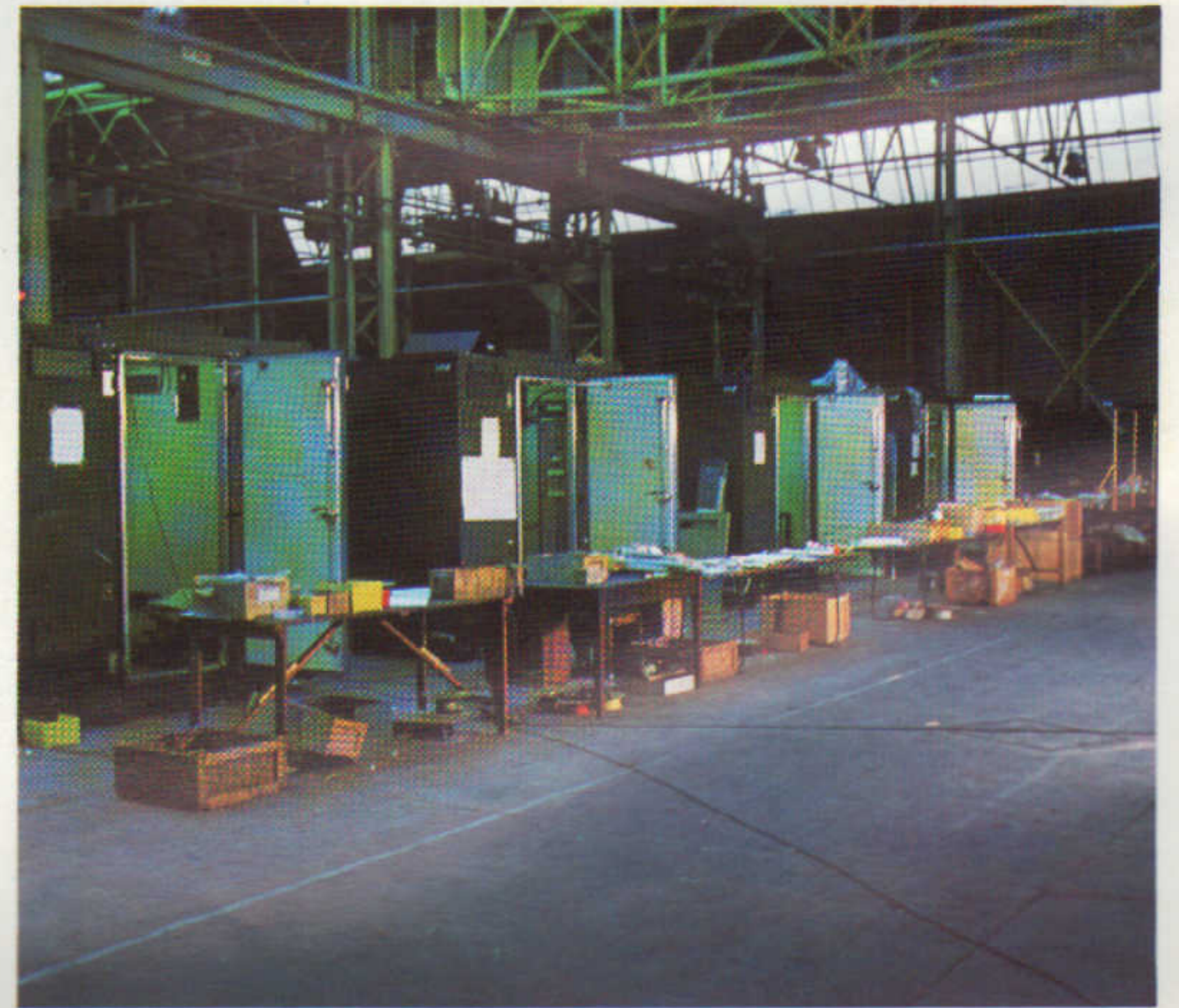
S600 Cabins being assembled at Marconi Radar Systems' Crompton Works
