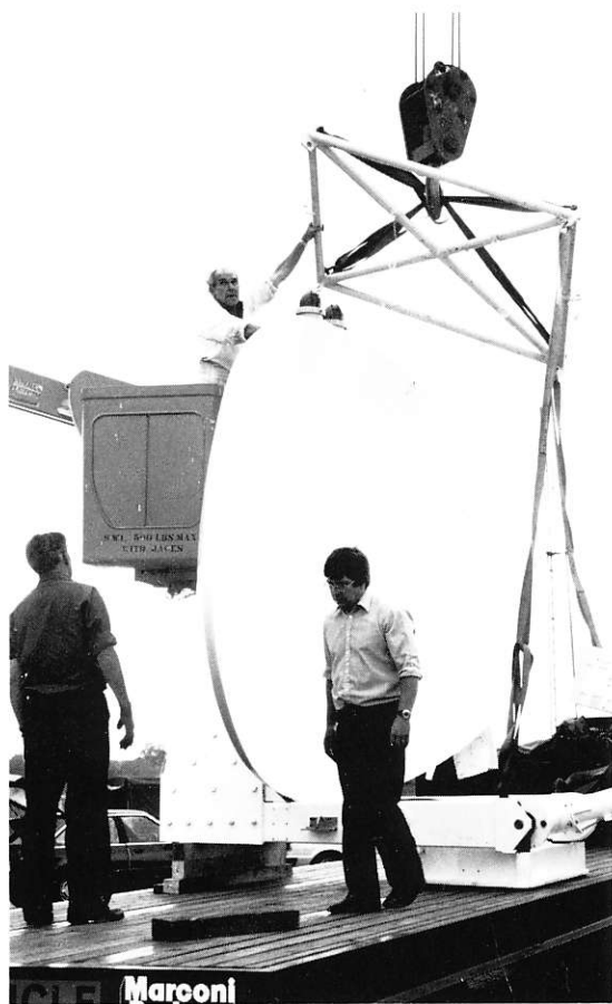
The carbon fibre aerial complete with mounting arrangement being prepared for transit to the test site.
