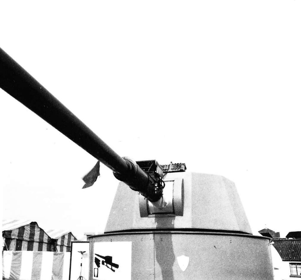
On show outside at Whale Island was the 105mm Naval Patrol Gun MK 1. The system design of the gun combines the expertise of the Royal Ordnance Factory, Nottingham, and Marconi Radar at Leicester, supported by specialist sub-contractors. The gun is fitted with equipment derived from the Marconi SFCS600 Fire Control System in conjunction with a periscopic sight with built-in laser rangefinder.
