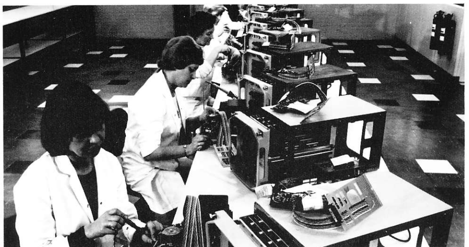
Assembling Gun Control Cubicles at Gateshead Works.
