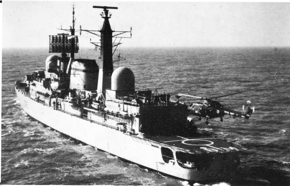
ABOVE: this view of HMS Sheffield clearly shows the two radomes housing the Type 909 (Sea Dart) tracker radars.
