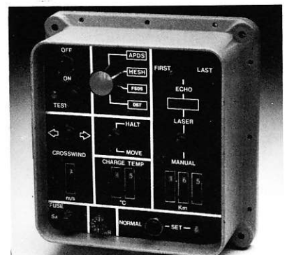
Commander's Control Panel for our SFCS600 tank fire control system.
