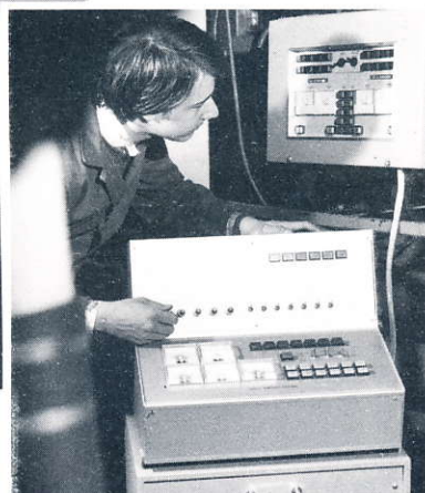
BELOW: Marconi control equipment for the chilled air plant of a nuclear submarine on trial at York Borg Warner.
