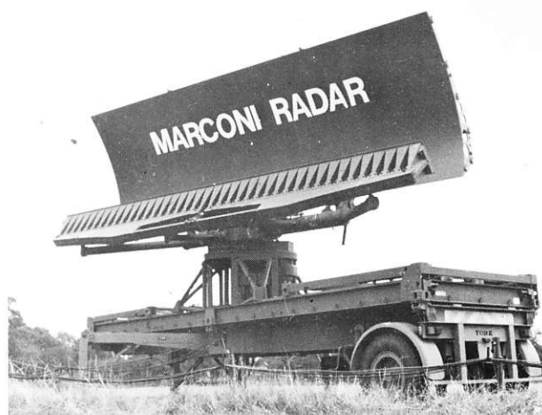
This S1061 antenna, shown here ready for display at Farnborough, is similar to the one we are supplying to the CAA for the South Shetlands.
