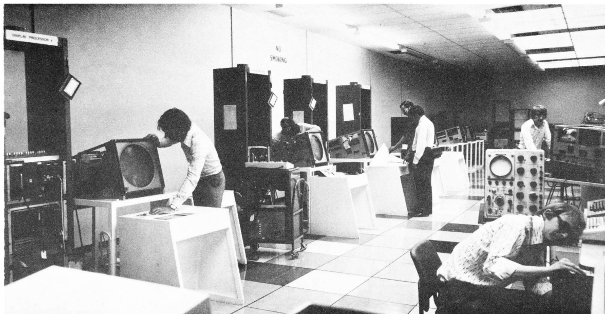
S.3017 Display complex driven by Locus 16's being tested in the Pre-Commissioning Test area at Writtle Road Works. 33 of these computers and displays are to be installed at the Scottish Air Traffic Control Centre.
