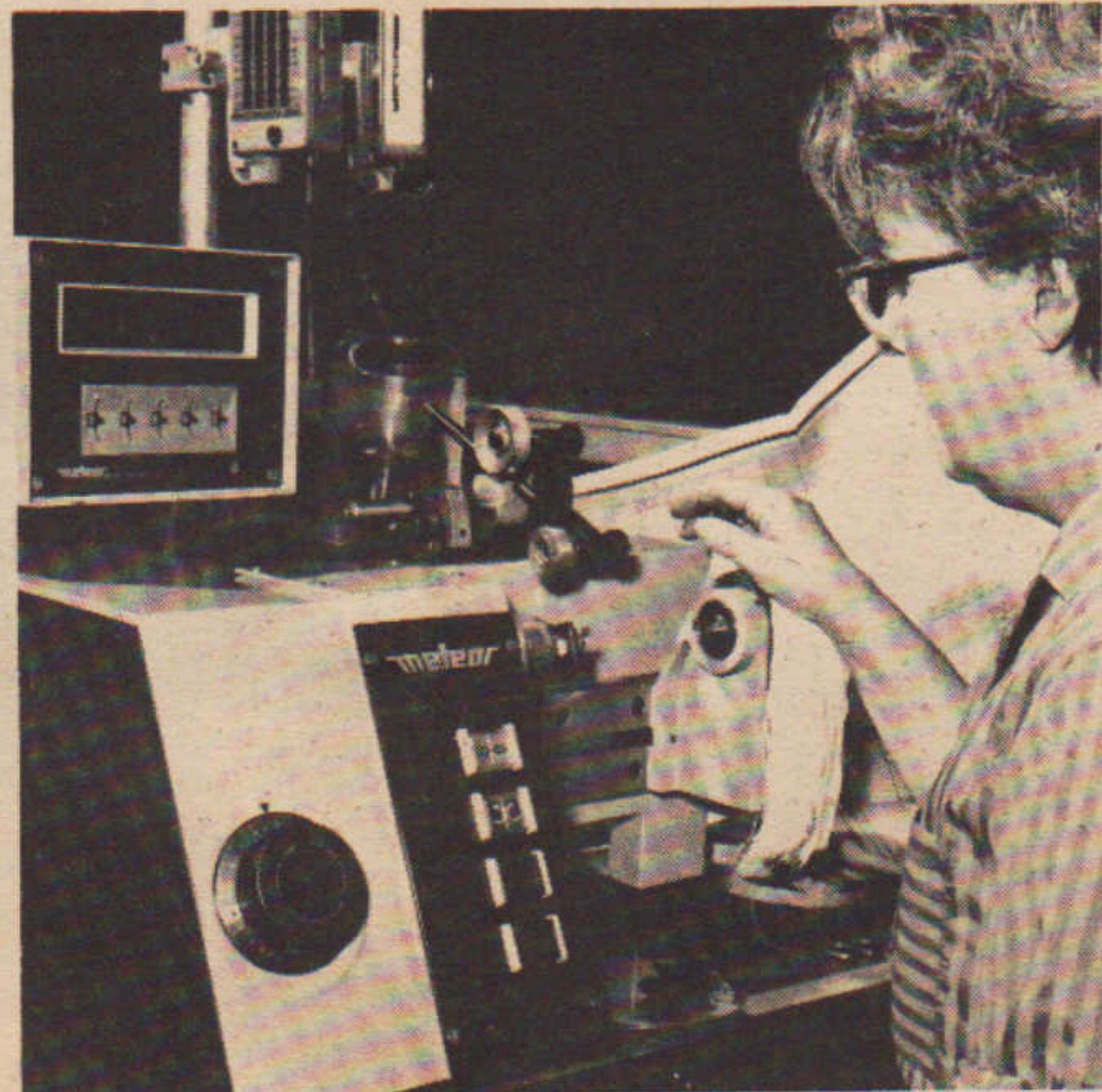
Mrs. A. Frost, coil winder, winding transformer coils for use in 6402 aero units.
