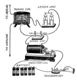
Simple spark-gap transmitter, typical of low power transmitters homebuilt by amateurs to explore the exciting new technology of radio Source: Seton E.T. (1917) The Woodcraft Manual for Boys, Doubleday, Page & Co., New York
