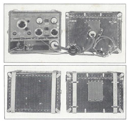
Above: Type PRS1 Transmitter-Receiver set coupled with Power Supply Unit Below: Type PRS1 in closed carrying cases, ready for transportation Source: Jacques Hamel, Contrecœur
