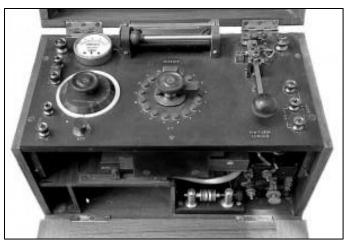
Wireless Telegraphy (W/T) Trench Set 50 Watt D.C. (also known as the BF set). The spark gap is clearly seen at the bottom Source: Thrower, K., ``Army radio communication in the Great War``
