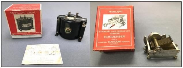
Distortionless Transformer and Straight Line Frequency Condenser, Canadian Marconi Company (1925-1929) Source: Ultra TCS collection
