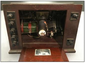
Marconiphone Model 1, inside view showing the single UV-201 valve Source: Ultra TCS collection, on loan from École de technologie supérieure-ETS (Donation R. Mc Duff)
