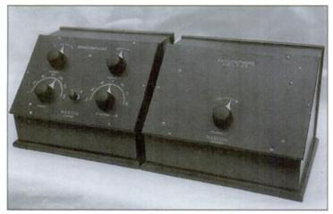
Marconiphone Model 1 (Mk I) with its two-valve audio amplifier Source: Murray R.P. (2005) "The Early Development of Radio in Canada, 1901-1930"
