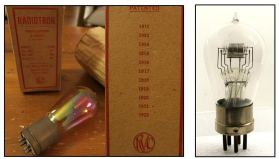
On the left, the UV-202 Radiotron 5 Watts Power output triode (1922); on the right, the Bower Electric K-4 four electrode valve with its 2 grids clearly visible (1924) Source: Ultra TCS collection
