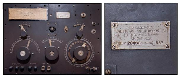
Type 2846B Maritime Receiver; originally designed as a crystal receiver in 1918 and 1920; later converted to vacuum tubes (ca.1925). It may have kept its crystal detector as a back-up mode Source: Musée Québécois de la Radio, Sorel-Tracy
