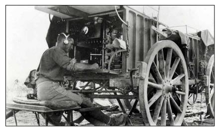
One of the first tactical transmitter-receiver set made by Marconi UK, with its Royal Engineers Signal Service operator (1500W transmitter version) Source: www.royal-signals.org.uk
