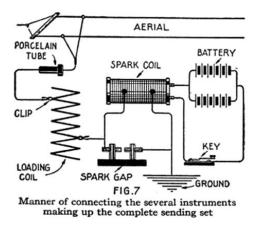
Schematic of an amateur spark transmitter using an automobile type inductance "spark coil" Source: Popular Science Magazine, October 1916
