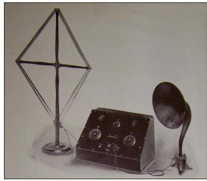
Marconiphones (here a Model III) could be used with a 60 or 120 ft long external antenna or with a loop antenna for use inside buildings Source: Company catalog, ca. 1925, Musée Québécois de la Radio, Sorel-Tracy
