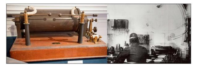
Left: Spark Transmitter Model 1216, S/N 007, Marconi Wireless Telegraph Company of Canada, 1907 Right: The Titanic radio room on its last trip with a similar Marconi transmitter (April 1912)<sup>16</sup> Source: Musée Québécois de la Radio, Sorel-Tracy<sup>17</sup>
