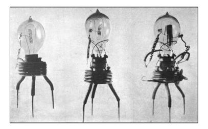
**The first prototype Fleming valves, built October 1904** Source: Fleming J.A. (1919), ``The Thermionic Valve and Its Developments``, Wireless Press
