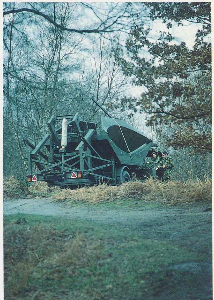
TACTROP antenna in the stowed position
