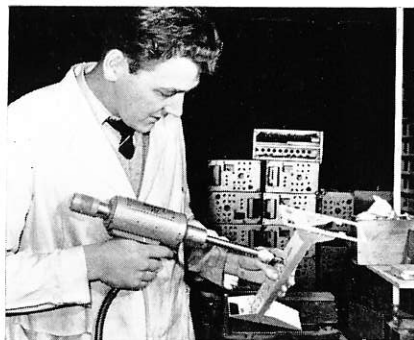
At work at Basildon on the chassis sub-assembly for the AD 308 (radio teletype) is Vic Warren, Sheet Metal Shop. He is seen here using a Chobert riveting gun
