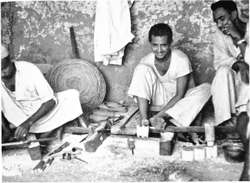
Craftsmen in Khartoum turn bangles and bracelets in ivory on lathes of their own design. The mandrel is turned with a bow in the right hand and one turn of string on the mandrel, while the tool is worked with the feet and the left hand. Dennis Fletcher of Broadcasting took this picture when he was in the Sudan
