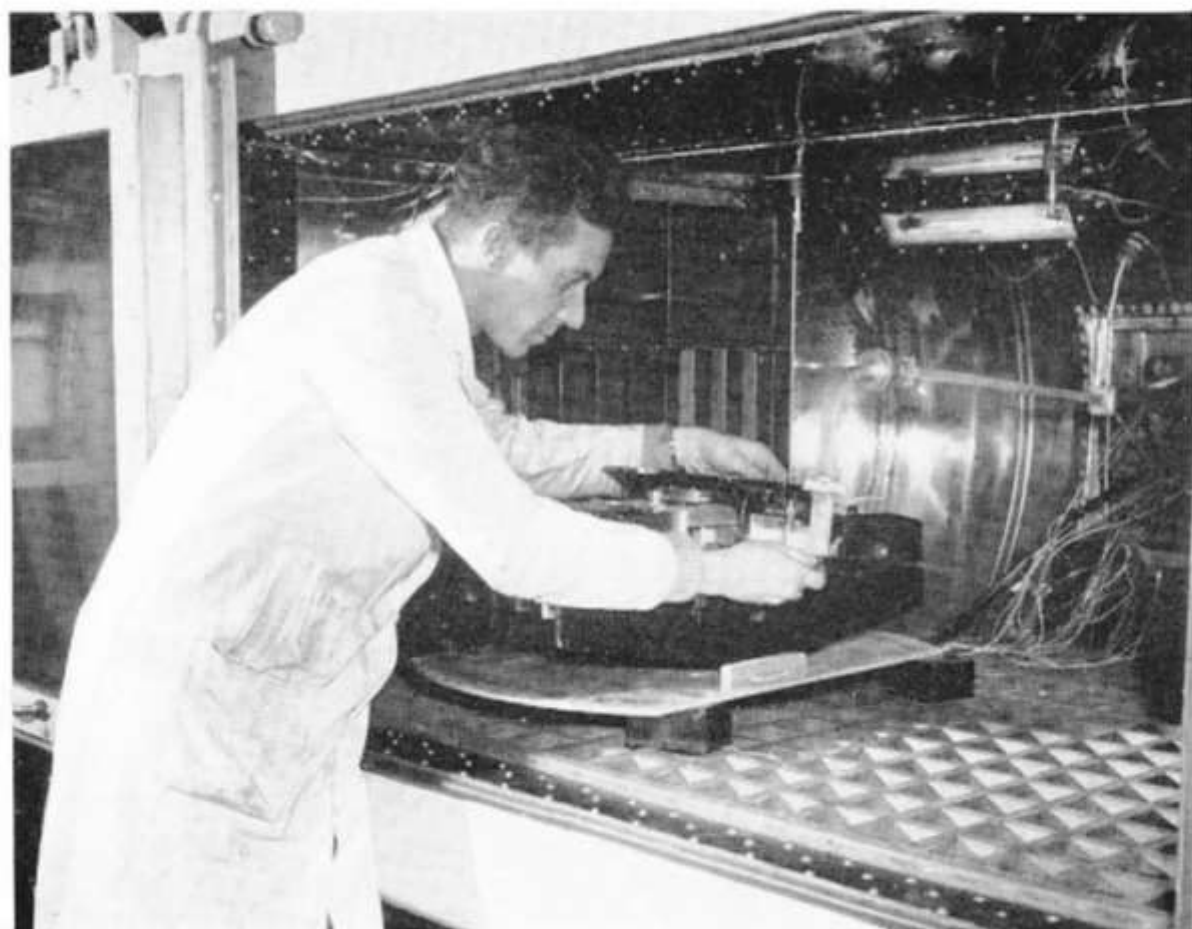
BELOW: This three-ton climatic test chamber, of which only about five exist in this country, was formerly at New Street and is now installed in Aeronautical Division's Environmental Test Laboratory. It is capable of simulating any sort of atmospheric condition. H. Waller, in charge of Environmental Test, is about to check the performance of a doppler AD2300 under conditions of extreme cold
