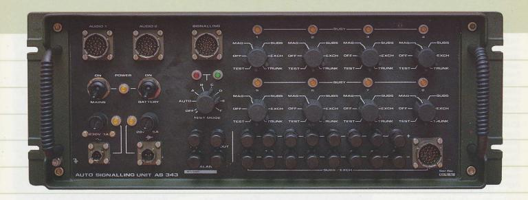
Whilst a MUX983 multiplexer can interface with a number of telephone systems such as magneto and 2 and 4 wire E&M systems, the CLAYMORE Automatic Signalling Unit greatly enhances the flexibility of a system.
