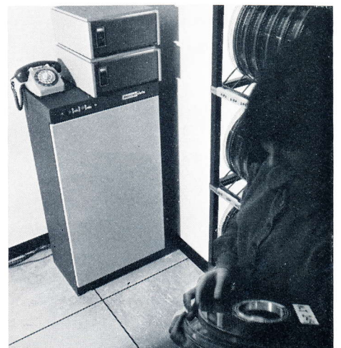
Marconidata H6010 Series data transmission equipment.
