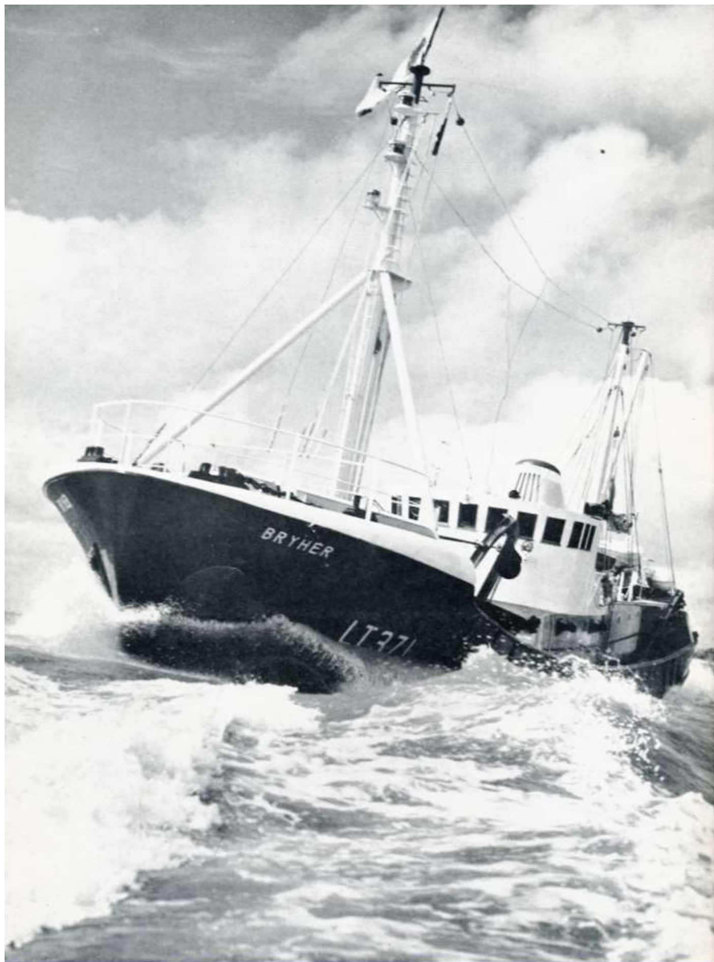
Trawlers go out from east coast ports and work in appalling weather to bring home our fish. This is Bryher from Lowestoft which carries Marconi Marine equipment to help her on her way. Owned by W. H. Podd Ltd. and built by Brooke Marine, she is fitted with a Gannet II transmitter, a Guardian receiver, a DF loop and a Graphette echo sounder [Dowsett Holdings Ltd.]
