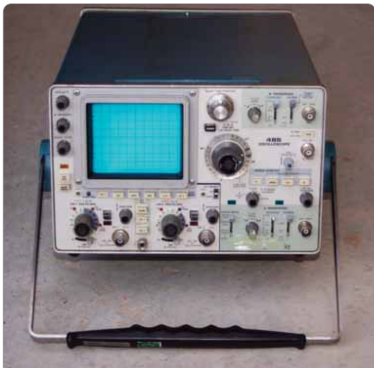
Figure 1: Example of an analog oscilloscope: Tektronix's model 485, a 350MHz, dual-channel instrument that debuted in 1973
