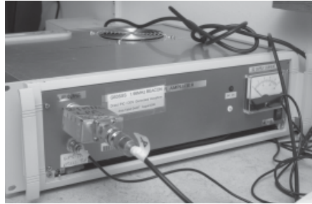
Fig. 3. Andy Talbot's 1960 KHz Beacon transmitter, operational. (Photo Steve Nichols, G0KYA).
