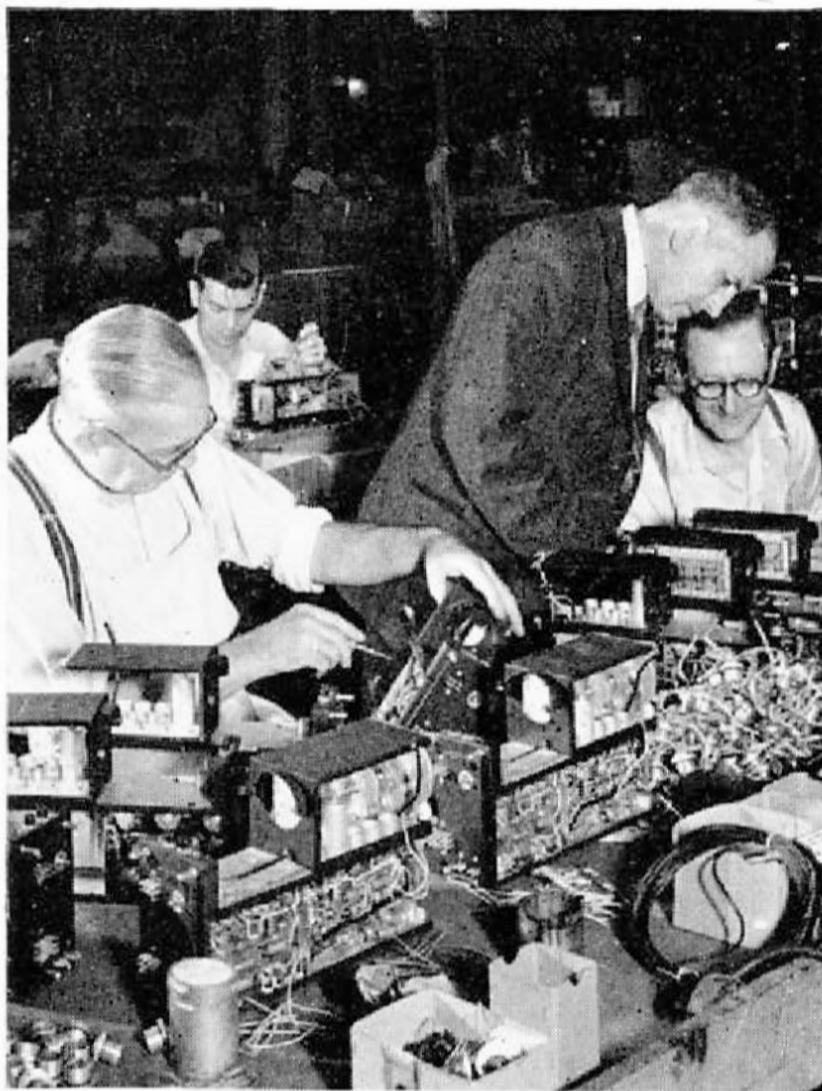
Above: wiring plugs for master controllers of automatic direction-finding equipment, Bill Wisbey, A. J. Burnell (Foreman), and Johnny Evans (Inspector)
