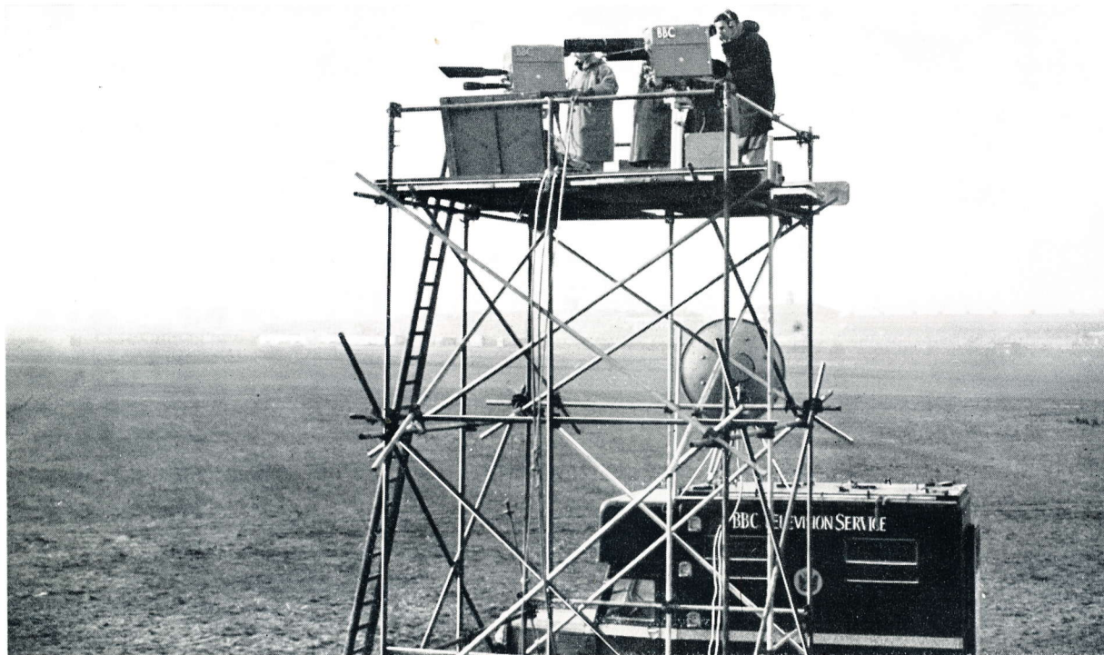
Marconi cameras and centimetric links being used by the BBC at a race meeting
