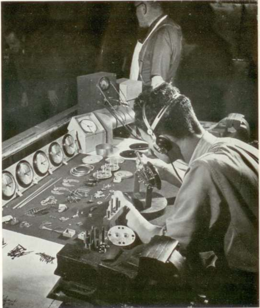
An instrument maker at work on clocks for high precision frequency measuring equipment.
