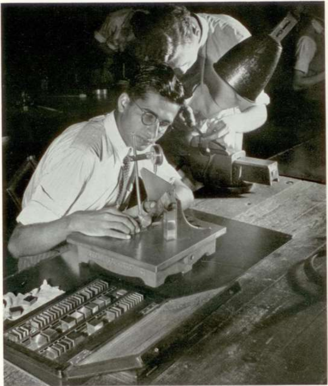
An Indian graduate apprentice at work with sine bar and slip gauges in the Apprentices Training Centre.
