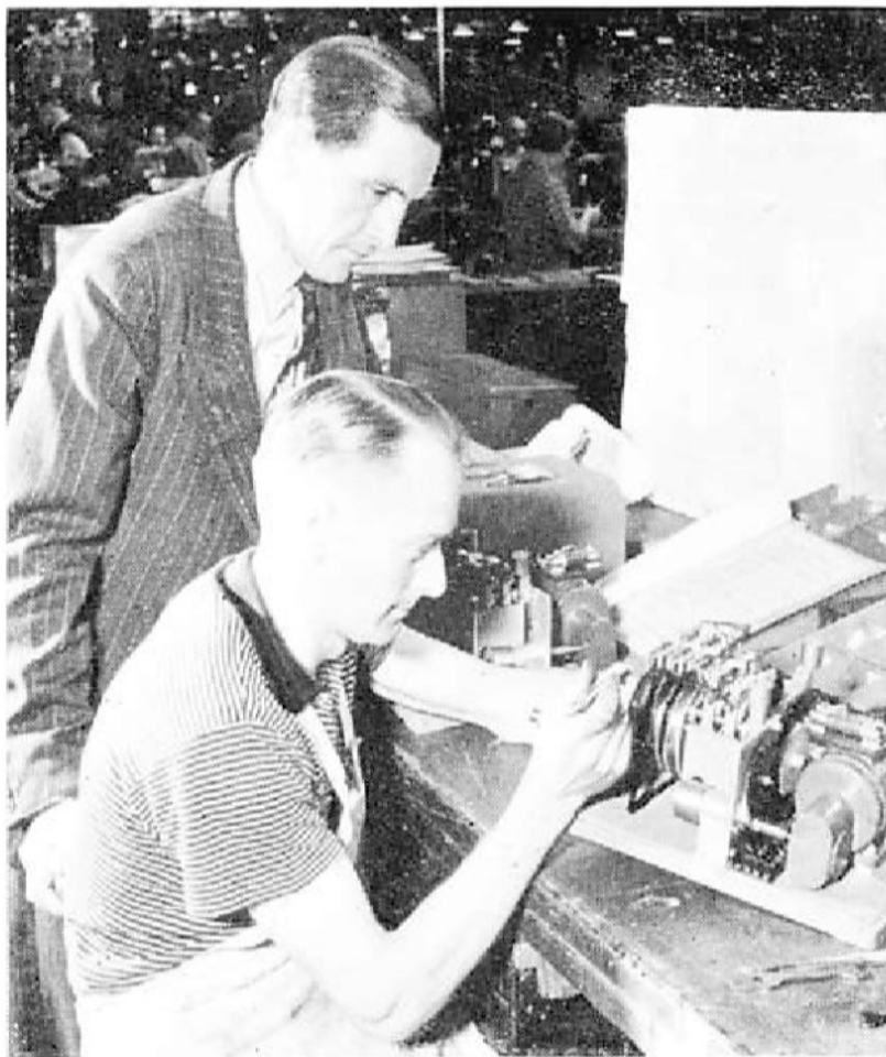
Setting the contacts of the code sender of an RB.109 radio beacon. Jack Stock, Foreman, Section 15, and Ron Bright
