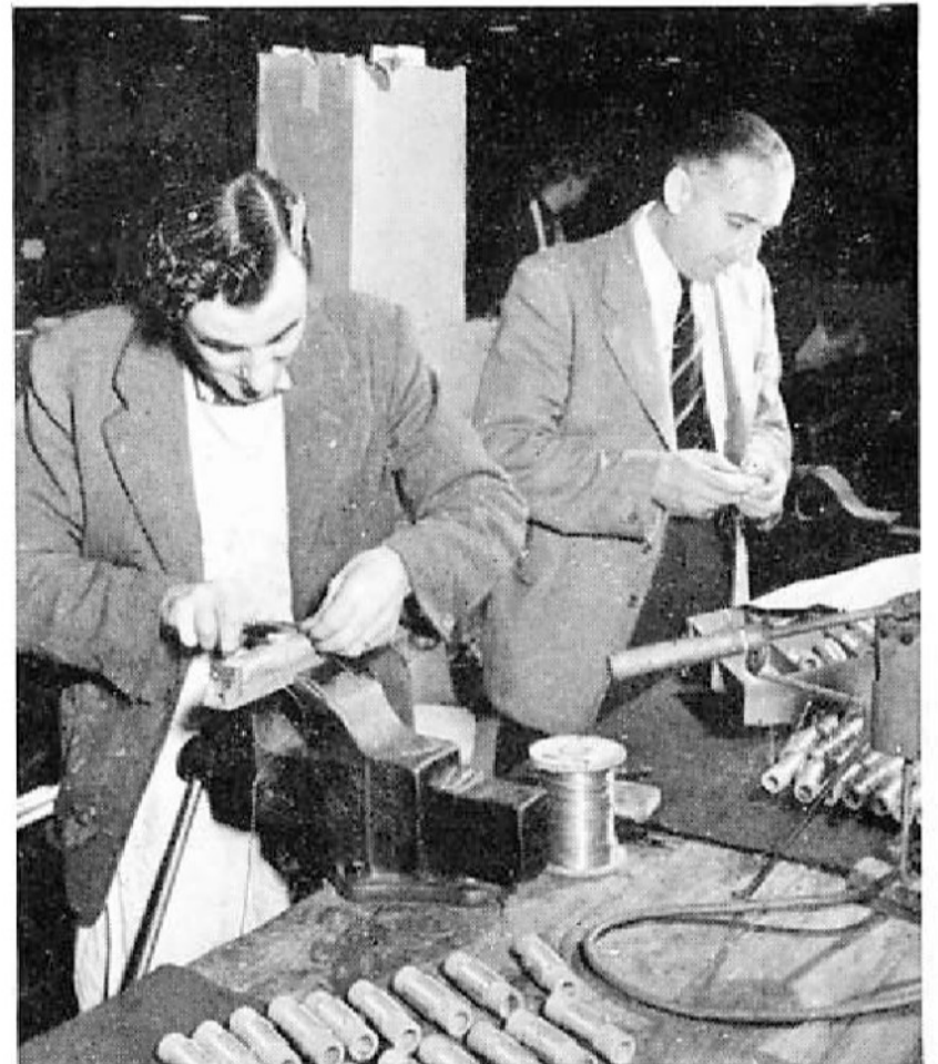
Bill Walden, chargehand (right), inspecting coils for an aircraft transmitter wound by Stan Perry
