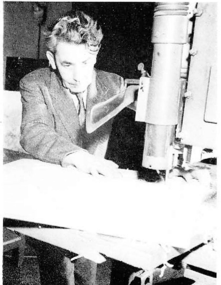
A fret for a loudspeaker cabinet being cut to a master by Ralph Guy with a very high speed routing machine.
