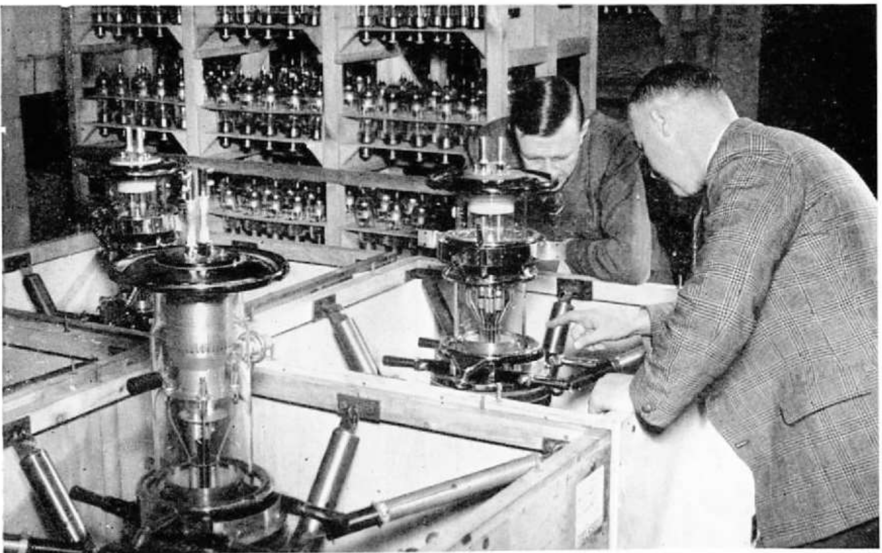
Valves for the B.B.C. Types CAT 14 and 17 going through Valve Test. Discussing the CAT 17 are N. W. Jenkins, Valve Section, and J. P. Baker, Valve Test
