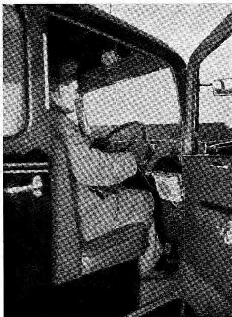
Marconi equipment on the first radio-equipped taxicab. The microphone is just above the driver's head and the Marconi type H16 V.H.F. transmitter/receiver is installed beneath the driver's seat.
