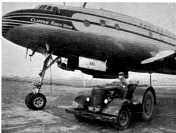
A Pan American World Airlines System tractor fitted with Marconi H18 V.H.F. radio.
